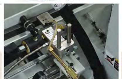
Aligns sticks precisely to the edges of the core
