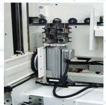
Vertical spindle shaper with stacked tooling to reduce setup
