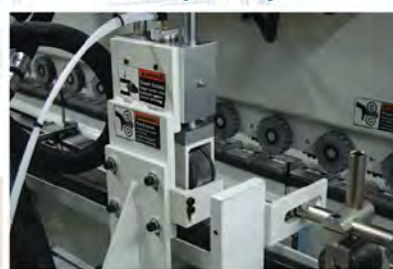
Optional No-Drip Stick System with pneumatic clamping
