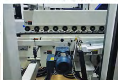
Stick feed drive motor(s) automatically aligns and feeds build-down and scribe sticks onto the bottom of the core
